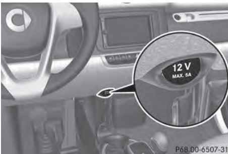
Auxiliary power outlet
