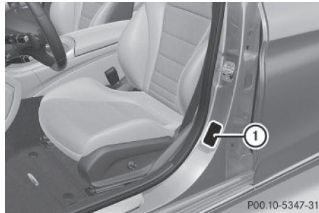
Location of vehicle identification plate (example, left-hand-drive vehicle)
