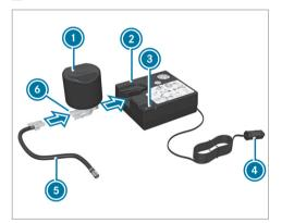
Pull plug 4 with the cable and hose 5 out of the tire inflation compressor housing.
