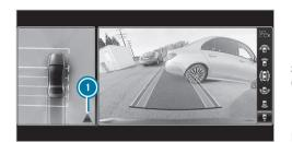
Vehicles with Blind Spot Assist: Cross Traffic Alert can warn drivers of any crossing traffic when backing up out of a parking space. The radar sensors in the bumper also monitor the area adjacent to the vehicle. If a critical situation is detected, symbol 1 appears in the media display. If the driver does not respond to the warning, the vehicle's brakes can be applied automatically.
