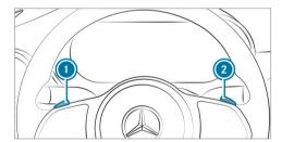
When the automatic transmission is shifted to position D, you can manually shift it with the steering wheel gearshift paddle. If permitted, the automatic transmission shifts to a higher or lower gear depending on the steering wheel gearshift paddle being pulled.
