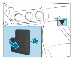
Open cover in the direction of the arrow and remove it.
