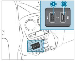
Example: USB ports in the rear passenger compartment center console
