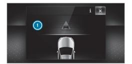
If autonomous braking or situation-dependent braking assistance has occurred, display ① appears in the multifunction display and then automatically goes out after a short time.
