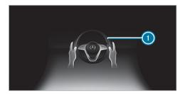
If the system detects that the driver has not steered the vehicle for a considerable period of time or has removed their hands from the steering wheel, an optical warning is given first. Display (a) appears in the multifunction display. If the driver still does not steer the vehicle, or gives no confirmation to the system, a warning tone sounds in addition to the visual warning message.
