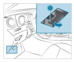
▶ To open: pull lever ① to release the hood.
