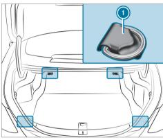
Tie-down eyes (vehicles with through-loading feature in the rear bench seat)
