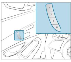
Set the seat, the steering wheel, the Head-up Display and the outside mirrors to the desired position.
