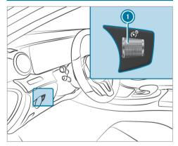
Turn brightness control 1 up or down. The lighting of the Instrument Display and in the control elements of the vehicle interior is adjusted.
