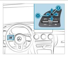
The on-board computer is operated using left-hand Touch Control ② and left-hand back/home button ①.
