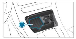
Place the mobile phone as close to the center of mat ① as possible with the display facing upwards.
