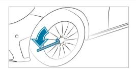
Using the lug wrench, loosen the wheel bolts on the wheel you wish to change by about one full turn. Do not unscrew the bolts completely.
