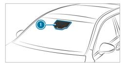
Traffic Sign Assist detects traffic signs with multifunction camera 1. It assists you by displaying detected speed limits and overtaking restrictions in the instrument cluster and optionally in the head-up display or central display.
