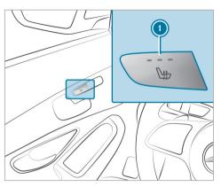
➤ To switch on/increase the level: press button ① repeatedly until the desired heating level is set.
