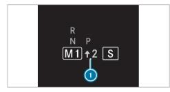
If gearshift recommendation message (1) is shown on the multifunction display, shift to the recommended gear.
