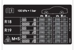
Some tire pressure tables only show the rim diameter instead of the complete tire size, e.g. **R18**. The rim diameter is part of the tire size and can be found on the tire side wall ( $\rightarrow$  page 410). Be sure to also observe the following further related subjects:
