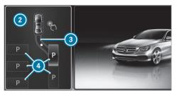
The media display shows the view of Active Parking Assist. Area 2 displays detected parking spaces (4) and vehicle path (3).
