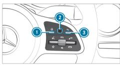
Operate the multimedia system with Touch Control 2 and associated buttons 1 and
