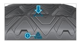
Six marks show where the bar indicators (arrow) are integrated into the tire tread. They are visible once a tread depth of approximately 1/16 in (1.6 mm) has been reached.
