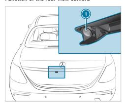
When you engage reverse gear, the image from rear view camera (1) is shown in the multimedia system. Dynamic guide lines show the path the vehicle will take with the steering wheel in its current position. This helps you to orient yourself and to avoid obstacles when backing up.
