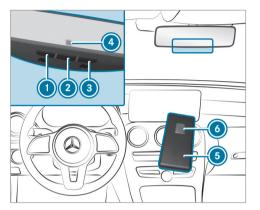
Check if the transmission frequency of the remote control has the frequency range of 280 to 868 MHz.
