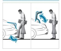
With HANDS-FREE ACCESS you can open, close or interrupt trunk lid movement by performing a kicking movement under the rear bumper.
