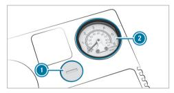
To reduce the tire pressure: press pressure release button 1 next to pressure gauge
