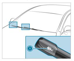
Remove protective film (1) from the maintenance display on the tip of the newly installed wiper blades.
