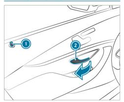
➤ To unlock and open a front door: pull door handle ②. Locking pin ① pops up when the door is unlocked. To unlock a rear door: pull the rear door handle.
