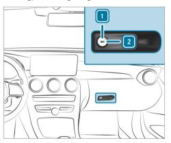
Turn the emergency key a quarter turn clockwise 2 (to lock) or counter-clockwise 1 (to unlock).
