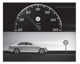
If a change in the speed limit is detected and automatic adoption of speed limits is activated. the new speed is automatically adopted as the stored speed ( $\rightarrow$  page 220).
