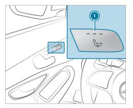
To switch on/increase the level: press button (1) repeatedly until the desired ventilation level is set. Depending on the ventilation level, up to three indicator lamps will light up.
