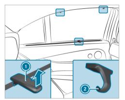
Pull the roller sunblind out by tab (1) and hook it onto brackets 2 at the top of the window.
