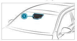
Active Lane Keeping Assist monitors the area in front of your vehicle by means of multifunction camera ①. It serves to protect you against unintentionally leaving your lane. You will be warned by vibration pulses in the steering wheel and guided by a course-correcting brake application back into your lane.
