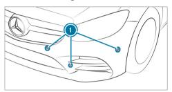
Parking Assist PARKTRONIC is an electronic parking assistance system with ultrasound. It monitors the area around your vehicle using multiple sensors ① on the front bumper and on the rear bumper. Parking Assist PARKTRONIC shows you the distance between your vehicle and a detected obstacle visually and audibly.
