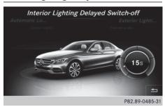
The interior lighting is activated for the duration of the delayed switch-off time when the key is removed from the ignition lock.
