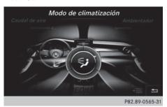
Setting the climate mode (airflow setting) determines the airflow. The setting is only active when the air-conditioning system is set to "AUTO".
