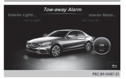
An audible and visual alarm is triggered if your vehicle's angle of inclination is altered while the tow-away alarm is armed. This can occur if the vehicle is jacked up on one side, for example.
