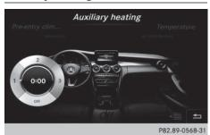
You can pre-set three departure times for automatic activation of the auxiliary heating. Selecting the pre-set time:
