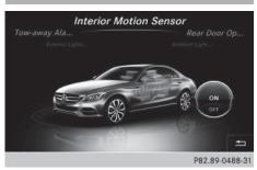
When the interior motion sensor is armed, a visual and audible alarm is triggered if movement is detected in the vehicle interior. This can occur if someone reaches into the vehicle interior without authorization, for example.
