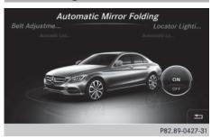
When the Automatic Mirror Folding function is activated, the exterior mirrors fold in automatically as soon as you lock the vehicle from the outside. The exterior mirrors fold out automatically again as soon as you unlock the vehicle.
