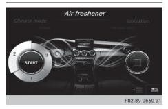
The perfume atomizer makes it possible to scent the air in individual compartments in the vehicle interior. Further information (see the vehicle Operator's Manual).
