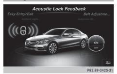
You can also set an audible signal to confirm that the vehicle has been locked.
