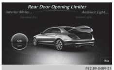
Activating the trunk lid opening height restriction allows you to avoid bumping the trunk lid on a low garage ceiling, for example.
