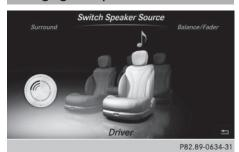
Select Sound Source specifies which seatbased media source shall be output on the speaker system.
