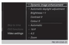
► To activate or deactivate: check or uncheck the box in front of Dynamic Image Enhancement.
