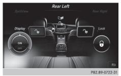
This function serves to switch the rear-compartment displays on/off.
