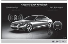
You can also set an audible signal to confirm that the vehicle has been locked.
