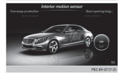
When the interior motion sensor is armed, a visual and audible alarm is triggered if movement is detected in the vehicle interior. This can occur if someone reaches into the vehicle interior without authorization, for example.
