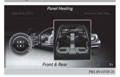
The panel heating function warms the surfaces with which the vehicle occupants frequently come into contact. Activation of the panel heating using COMAND as described below only works if seat heating is activated (see the vehicle Operator's Manual).
