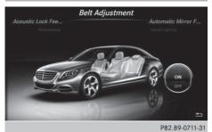
The seat-belt adjustment function adjusts the driver's and front-passenger seat belt to the upper body of the occupants.
