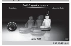
Select Sound Source specifies which seatbased media source shall be output on the speaker system. Example: a media source is being listened to using headphones in the left-hand rear seat.
