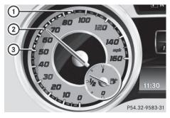
Example: DISTRONIC PLUS displays in the speedometer
