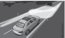
You can use this function to set the headlamps to change between low beam and high beam automatically. The system recognizes vehicles with their lights on, either approaching from the opposite direction or traveling in front of your vehicle, and consequently switches the headlamps from high beam to low beam.
