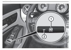
▶ To enable/disable: press button ①. If indicator lamp ② is lit, operation of the rear side windows is disabled. Operation is only possible using the switches in the driver's door. If indicator lamp ② is off, operation is possible using the switches in the rear compartment.
