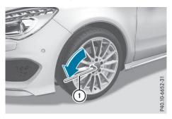
► Using lug wrench ①, loosen the bolts on the wheel you wish to change by about one full turn. Do not unscrew the bolts completely.
