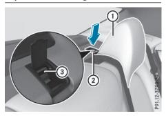
The Top Tether anchorage points are installed in the rear compartment behind the head restraints on the parcel shelf.
