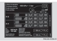
Some tire pressure tables show only the rim diameters instead of the full tire size, e.g. **R18**. Rim diameter is part of the tire size and can be found on the tire sidewall
