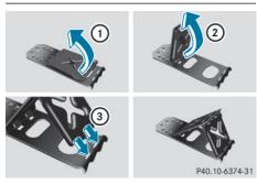
If your vehicle is equipped with a wheel chock, it can be found in the tire-change tool kit (> page 234).
