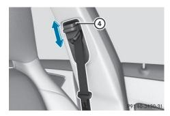
The shoulder section of the seat belt must always be routed across the center of the shoulder. Adjust the belt outlet if necessary.
