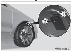
You must remove the cover of the front wheel housing before you can change the front turn signal lamp.
