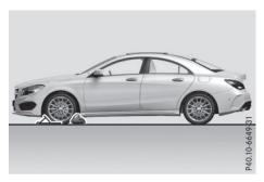
Securing the vehicle on level ground
