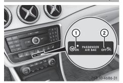
PASSENGER AIR BAG ON indicator lamp (1) and PASSENGER AIR BAG OFF indicator lamp (2) are part of the Occupant Classification System (OCS).
