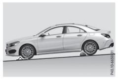
Securing the vehicle on slight downhill gradients
