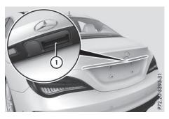
► To unlock the trunk lid: pull the handle on the trunk lid.
