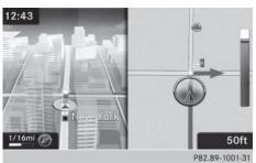
Before and during a change of direction, the map is shown on the left side of the display and a view of the intersection or a 3D image on the right. Lane recommendations (white directional arrows) may be shown at the bottom of the display for multilane roads.
