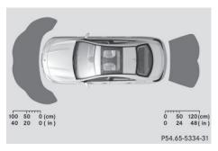
If there is an obstacle within this range, the relevant warning displays light up and a warning tone sounds. If the distance falls below the minimum, the distance may no longer be shown.
