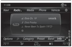
To select Info in the radio menu bar: turn and press the controller. Information on the currently received program is displayed.
