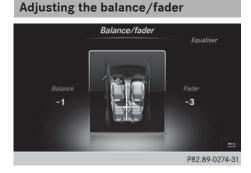
Balance moves the focus of the sound between left and right.
