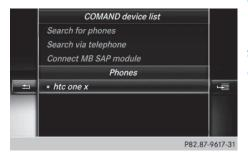
To select a mobile phone from the device list: turn the controller and press to confirm.
