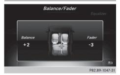
Balance adjusts the volume left and right. Fader adjusts the volume in front and rear. For the best sound, setting 0 is recommended.
