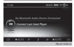
During the search for mobile phones, the connection with the Bluetooth® audio device is terminated (▷ page 136). In the Bluetooth® audio basic display (▷ page 224) you will see the No Bluetooth Audio Device Connected message and the Connect Last Used Player menu item cannot be selected.
