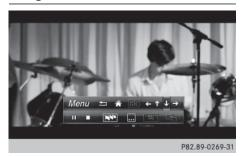
► In full-screen mode, press the controller The DVD functions menu is shown.
