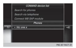
► To select a mobile phone from the device list: turn and press the controller. If the mobile phone supports the Bluetooth® PAN profile or the USB classes RNDIS, CDC/NCM or CDC/ECM, Internet access is set up. You can use the Internet functions.
