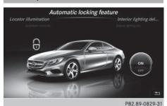
When the automatic locking feature is activated, the vehicle is locked automatically when the ignition is switched on and the vehicle is traveling faster than walking pace.
