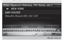
The keyword search is used to help find destinations using fragments of words. If you enable the appropriate setting in the search options, the keyword search is tolerant of errors ( $\triangleright$  page 73).
