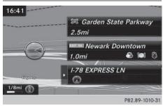
Requirement: the Highway Information map content must be enabled (▷ page 100). While driving on the highway, gas stations, rest stops, rest areas and highway exits are displayed along with their immediate distances from the current vehicle position.
