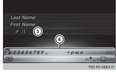
When the telephone number input line is selected, the character bar is adapted for entering digits.
