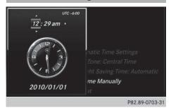
Vehicles with GPS reception: using the manual time settings, you can set the time forwards or backwards by up to several hours.
