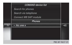
➤ To select a mobile phone from the device list: turn the controller and press to confirm. If the mobile phone supports the Bluetooth® PAN profile, Internet access is set up. You can use the Internet functions.
