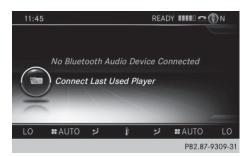
To confirm the Connect Last Used Player message in the basic display: press the controller.
