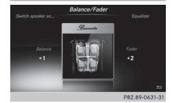
Balance moves the focus of the sound between left and right.
