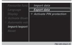
Vehicles equipped with a Garmin<sup>®</sup> MAP PILOT navigation module: if you want to import or export data using an SD card, you must first remove the Garmin<sup>®</sup> MAP PILOT SD card (⊳ page 85).
