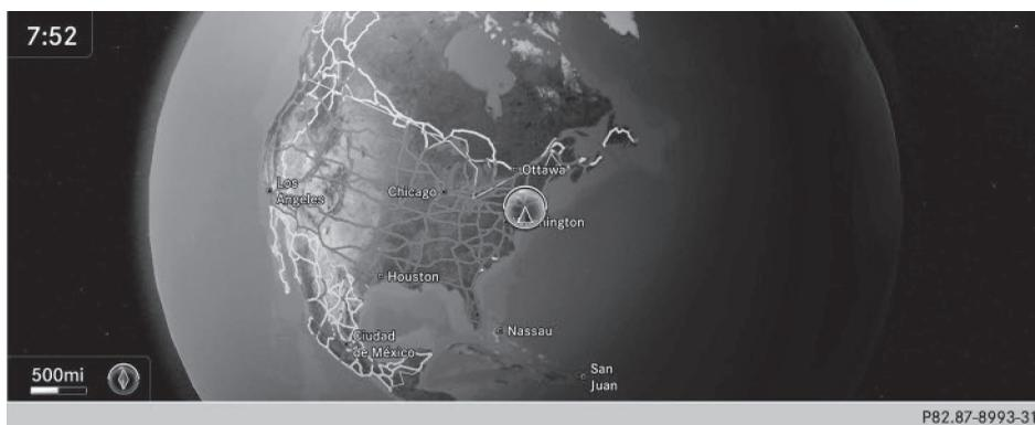
The navigation map and satellite images are shown in globe projection. This allows for a realistic map display free from distortion in all map scales.
