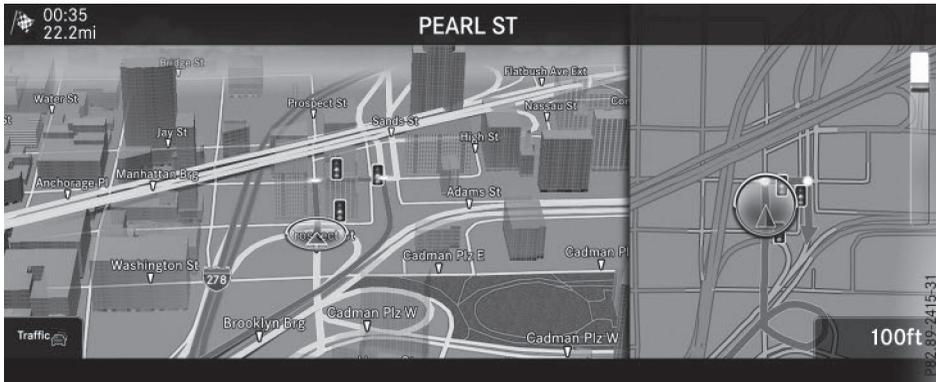
The change of direction is performed when the light-colored bar on the right drops down to 0 ft and the current vehicle position symbol has reached the white change-of-direction point.
