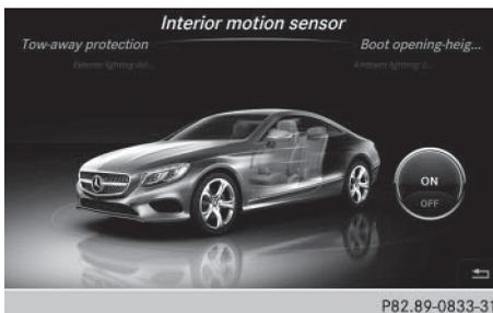
When the interior motion sensor is activated, a visual and audible alarm is triggered if movement is detected in the vehicle interior. This can occur if someone reaches into the vehicle interior without authorization, for example.
