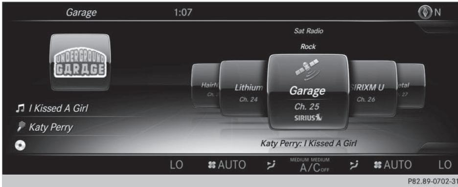
The additional display area occupies the left-hand or right-hand third of the display. The additional display area allows you to view various items of additional information. For instance, you can display an album cover in media mode or a permanent display, such as a small navigation map, in the additional display area.
