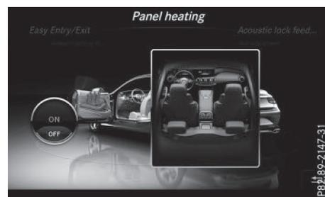
The panel heating function warms the surfaces with which the vehicle occupants frequently come into contact. Activation of the panel heating via the multimedia system as described below only works if seat heating is activated (see the vehicle Operator's Manual).
