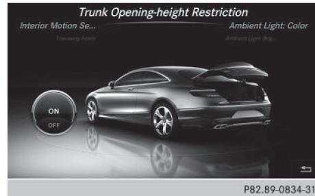
Activating the **Trunk Opening-height Restriction** function allows you to avoid bumping the trunk lid on a low garage ceiling, for example.
