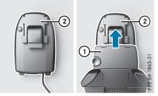
Slide smartphone cradle 1 onto contact plate 2 in the center console.
