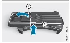
If the smartphone cradle is installed upright in the vehicle, the alignment plate can be adjusted for ease of use.
