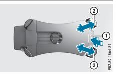
Press button ① on the smartphone cradle and at the same time push or pull both lower retainers ② into the desired position. The size of the smartphone cradle is adjusted.
