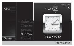
Using the manual time settings, you can set the time forward or back by up to several hours. ▶ Press the 🖾 button.
