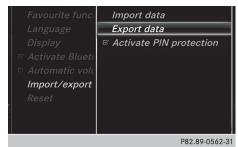
Vehicles equipped with a Garmin<sup>®</sup> MAP PILOT navigation module: if you want to import or export data using an SD card, you must first remove the Garmin<sup>®</sup> MAP PILOT SD card (> page 82).
