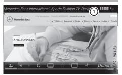
① Display of existing connection and signal strength of the mobile phone network
