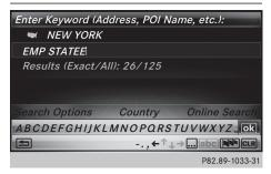
The keyword search is used to help find destinations using fragments of words. If you enable the appropriate setting in the search options, the keyword search is tolerant of errors (> page 60).
