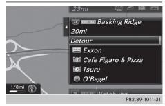
Highway information enables the use of the traffic jam function. The remaining route on the highway in this case is blocked in the direction of travel from the selected exit.
