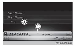
When the telephone number input line is selected, the character bar is adapted for entering digits.
