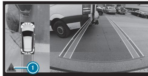
**Vehicles with Blind Spot Assist:** Drivers can also be warned of any crossing traffic when backing up out of a parking space. If a critical situation is detected, symbol **1** appears in the multimedia system display. If the driver does not respond to the warning, the vehicle's brakes can
