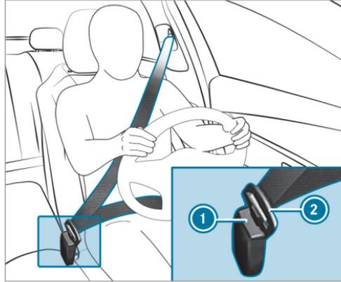
► Always engage seat belt tongue ② of the seat belt into seat belt buckle ① of the corresponding seat.
