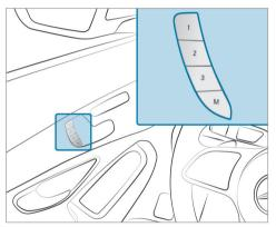
Set the seat, the steering wheel, the Head-up Display and the outside mirrors to the desired position.  Press memory button M and then press preset position button 1, 2 or 3 within three seconds.
