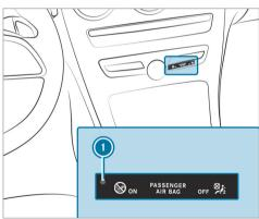
Indicator lamp 0 flashes when the ATA system is armed.
