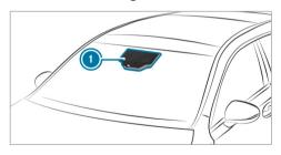
Traffic Sign Assist detects traffic signs with multifunction camera **()**. It assists you by displaying detected speed limits and overtaking restrictions in the instrument cluster and optionally in the head-up display or central display.
