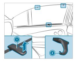
Pull the roller sunblind out by tab ① and hook it onto brackets ② at the top of the window.
