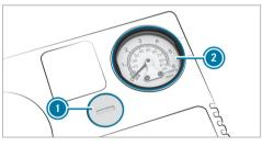
To reduce the tire pressure: press pressure release button () next to pressure gauge
