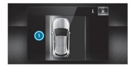
If a lane-correcting brake application occurs, display **()** appears in the multifunction display.
