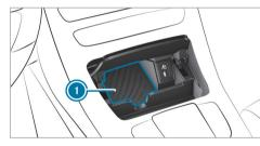
Place the mobile phone as close to the center of mat () as possible with the display facing upwards.
