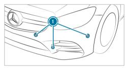
Parking Assist PARKTRONIC is an electronic parking assistance system with ultrasound. It monitors the area around your vehicle using multiple sensors () on the front bumper and on the rear bumper. Parking Assist PARKTRONIC shows you the distance between your vehicle and a detected obstacle visually and audibly.
