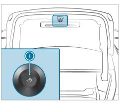
Press the emergency release button briefly. The trunk lid will unlock and open.
