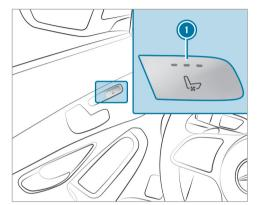
To switch on/increase the level: press button 1 repeatedly until the desired ventilation level is set. Depending on the ventilation level, up to three indicator lamps will light up.
