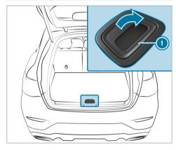
To open: lift the cargo compartment floor with handle (1) and fold it over at the hinge in the center of the cargo compartment floor.
