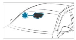
Active Lane Keeping Assist monitors the area in front of your vehicle by means of multifunction camera 1. It serves to protect you against unintentionally leaving your lane. You will be warned by vibration pulses in the steering wheel and guided by a course-correcting brake application back into your lane.
