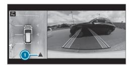
Vehicles with Blind Spot Assist: Cross Traffic Alert can warn drivers of any crossing traffic when backing up out of a parking space. The radar sensors in the bumper also monitor the area adjacent to the vehicle. If a critical situation is detected, symbol appears in the media display. If the driver does not respond to the warning, the vehicle's brakes can be applied automatically.
