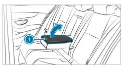
Press release catch (1) and swing the cover of the armrest upwards.
