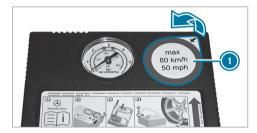
Remove sticker from the tire inflation compressor housing and affix it to the instrument cluster within the driver's field of vision.
