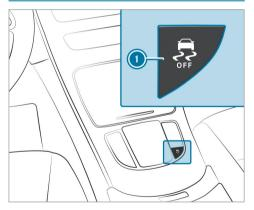
► To deactivate ESP®: press button ① until the ♣ ESP® OFF warning lamp lights up in
