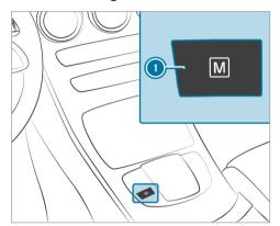
➤ To activate/deactivate: press button ①. Manual gearshifting is activated: transmission position M and the current gear appear in the multifunction display.
