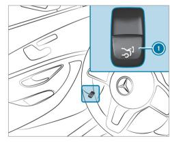
Pull remote opening switch for the tailgate.
