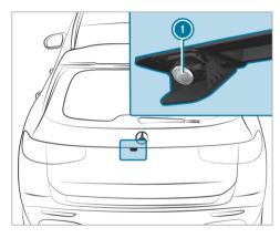
When you engage reverse gear, the image from rear view camera (1) is shown in the media display. Dynamic guide lines show the path the vehicle will take with the steering wheel in its current position. This helps you to orient yourself and to avoid obstacles when backing up.
