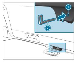
Insert emergency key 2 into opening 1 in the trim and push it in. The tailgate will be unlocked.
