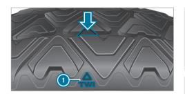
Six marks  $\bigcirc$  show where the bar indicators (arrow) are integrated into the tire tread. They are visible once a tread depth of approximately 1/16 in (1.6 mm) has been reached.
