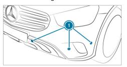
Parking Assist PARKTRONIC is an electronic parking assistance system with ultrasound. It monitors the area around your vehicle using multiple sensors on the front bumper and on the rear bumper. Parking Assist PARKTRONIC shows you the distance between your vehicle and a detected obstacle visually and audibly.
