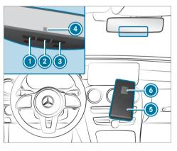
Check if the transmission frequency of the remote control has the frequency range of 280 to 868 MHz.
