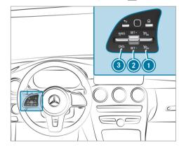
➤ To activate cruise control: press rocker switch ① up. To activate cruise control: press rocker switch 2 up (SET+) or down (SET-). The current speed is stored and maintained by the vehicle.
