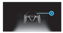
If the system detects that the driver has not steered the vehicle for a considerable period of time or has removed their hands from the steering wheel, an optical warning is given first. Display 1 appears in the multifunction display. If the driver still does not steer the vehicle, or gives no confirmation to the system, a warning tone sounds in addition to the visual warning message.
