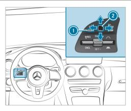
The on-board computer is operated using left-hand Touch Control ② and the left-hand back/home button ①.
