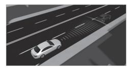
Active Distance Assist DISTRONIC maintains the set speed on free-flowing roads. If vehicles in front are detected, the set distance is maintained, if necessary, until the vehicle comes to a halt. The vehicle accelerates or brakes depending on the distance to the vehicle in front and
