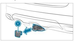
Remove cover 1 from the ball neck mount in the direction of the arrow.
