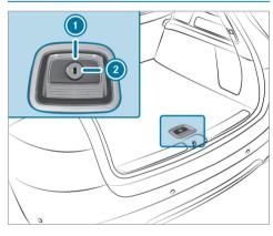
Turn the emergency key a quarter turn clockwise 2 (to lock) or counter-clockwise 1 (to unlock).
