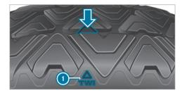
Six marks () show where the bar indicators (arrow) are integrated into the tire tread. They are visible once a tire tread depth of approximately  $V_{16}$  in (1.6 mm) has been reached.
