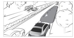
At speeds of at least 19 mph (30 km/h), a triangle that indicates a lane correction and its direction will be projected onto the road in the following cases:
