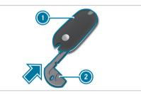
Press emergency key ② into the opening in the SmartKey in the direction of the arrow until cover ① opens. When doing so, do not hold cover ① closed.
