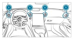
• To open or close: hold the center of air vent () and turn it to the left (open) or right (closed) as far as it will go. To set the airflow direction: hold the center of air vent () and move it up or down or to the left or right.
