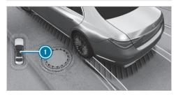
Display of Parking Assist PARKTRONIC (→ page 228) In the 3D view, left-/right-hand side of the vehicle, the virtual camera moves to the respective side of the vehicle. When you change the transmission position, the view is automatically adapted.
