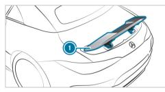
Rear wing () improves the driving stability of the vehicle and thus adapts the aerodynamics of the vehicle to the driving conditions.
