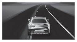
If the front wheel of the vehicle drives over a detected lane marking, this will be highlighted red in the Assistance menu in the driver's display.
