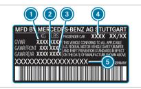
Vehicle identification plate (USA only) Maximum permissible gross vehicle weight Maximum permissible front axle load
