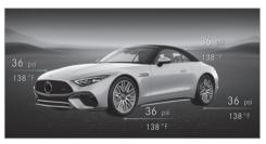
Tire pressure displayed after driving for a few minutes.: current values are not yet known to the system. The pressure/temperature values of each tire are displayed as soon as they are known to the system.
