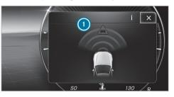
If autonomous braking or situation-dependent braking assistance has occurred, pop up appears in the driver's display and then automatically goes out after a short time.
