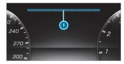
If the engine speed is too high or too low, you will not be able to change gears using the steering wheel paddle shifters. In this case, segments will light up red.
