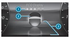
The ECO display shows an evaluation of your driving style on the driver's display depending on the situation. This enables you to check the efficiency of your driving style and adjust it if necessary. The ECO Display menu shows a ball (2) that will roll forwards or backwards on a stylized road in the direction of travel according to the driving characteristics.
