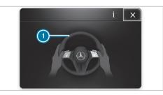
If the system detects that the driver has not steered the vehicle for a considerable period of time or has removed their hands from the steering wheel, an optical warning is given first. Display () appears on the driver's display. If the driver still does not steer the vehicle, or gives no confirmation to the system, a warning tone sounds in addition to the visual warning message.
