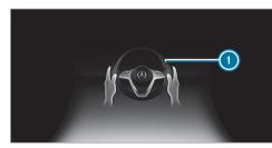
If the system detects that the driver has not steered the vehicle for a considerable period of time or has removed their hands from the steering wheel, display 1 appears. If the driver still does not steer the vehicle, a warning tone sounds in addition to the visual warning message.
