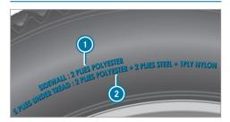
(i) The data shown in the image is example data. This information describes the type of tire cord and the number of layers in side wall (i) and under tire tread (ii).
