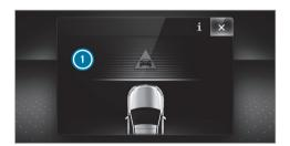
If autonomous braking or situation-dependent braking assistance has occurred, display will appear on the instrument display and then automatically go out after a short time.
