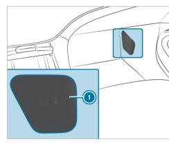
To open the fuse box: remove cover ①.
