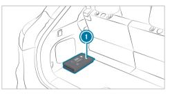
First-aid kit (soft-sided) () is located on the lefthand side of the cargo compartment in the asdelivered condition.
