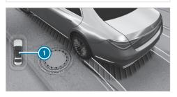
Display of Parking Assist PARKTRONIC (→ page 290) In the 3D view, left-/right-hand side of the vehicle, the virtual camera moves to the respective side of the vehicle. When you change the transmission position, the view is automatically adapted.
