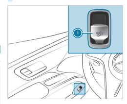
Pull remote operating switch ① until the tailgate opens.
