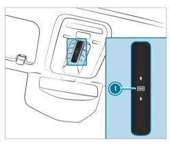
The sliding sunroof and the roller sunblind are operated using control panel ①.
