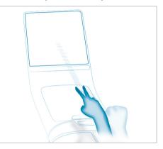
Implementation of the V-pose above the stowage compartment of the center console at the height of the central display
