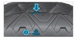
Six marks () show where the bar indicators (arrow) are integrated into the tire tread. They are visible once a tire tread depth of approximately  $V_{16}$  in (1.6 mm) has been reached.
