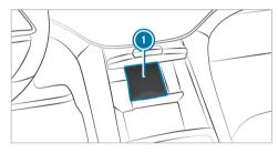
Example: wirelessly charging a mobile phone in the front stowage compartment (with MBUX Hyperscreen)
