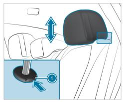
Push release knob ① in the direction of the arrow and pull out the head restraint.
