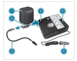
Pull plug ④ with the cable and hose ⑤ out of the tire inflation compressor housing.
