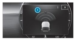
If autonomous braking or situation-dependent braking assistance has occurred, pop up appears in the driver's display and then automatically goes out after a short time.
