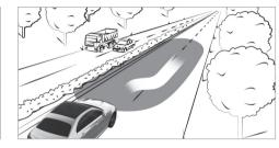
During assisted lane changes at speeds of at least 19 mph (30 km/h), the course of the lane change will flash.
