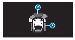
Optionally, obstacles detected by Parking Assist PARKTRONIC from a distance of approximately 3.3 ft (1.0 m) in front (2) and 2.2 ft (0.7 m) on sides (3) can also be displayed on the head-up display.
