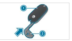
Press mechanical key ② into the opening in the key in the direction of the arrow until cover ① opens. When doing so, do not hold cover ① closed.
