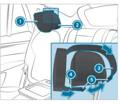
Guide long strap (a) of additional cushion (b) over head restraint (c) towards the rear of the vehicle.
