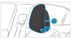
Take hold of the head restraint on both sides and press release knob ①.
