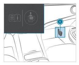
Remove flap ① of the fuse box in the front passenger footwell.
