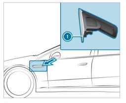
Press on the rear area of washer fluid filler flap
