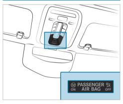
The PASSENGER AIR BAG indicator lamps display the status of the front passenger air bag.
