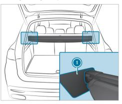
Insert the cargo compartment cover in brackets (1) on the left and right.
