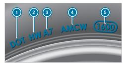
(i) The data shown in the image is example data. The TIN is a unique identification number to identify tires and comprises the following:
