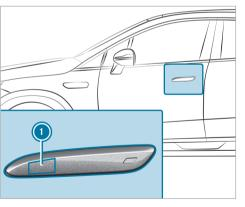
Locking and unlocking the vehicle with the NFC function Stop the digital vehicle key in the area of the NFC antenna ① on the door handle.
