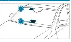
Radio-controlled equipment such as toll systems can be mounted only on areas () of the windshield that are permeable to radio waves.
