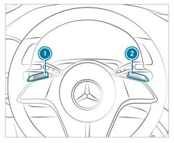
(i) When the vehicle is started again, **D** will automatically be set as the recuperation level.
