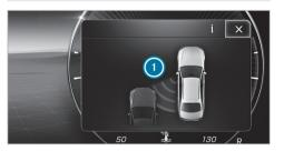
If a course-correcting brake application occurs, the red warning lamp flashes in the outside mirror and a warning tone sounds. In addition, a display indicating the danger of a side collision appears in the driver's display.
