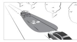
If you fall below the safe distance at speeds of at least 19 mph (30 km/h), a collision warning symbol will be projected onto the road.
