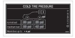
The tire pressure table shows the recommended tire pressure for all tires approved for this vehicle. The recommended tire pressures apply for cold tires under various operating conditions, i.e. loading and/or speed of the vehicle.
