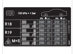
Some tire pressure tables only show the rim diameter instead of the complete tire size, e.g. **R18**. The rim diameter is part of the tire size and can be found on the tire side wall ( $\rightarrow$  page 433).
