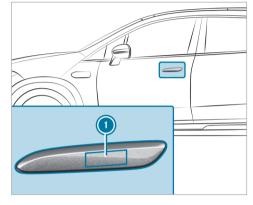
Extend the door handle: Touch the outer sensor surface.
