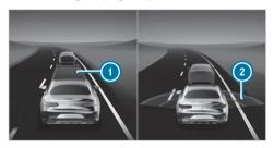
In the Assistance menu, an insufficient distance (1) to the vehicle in front is displayed in red. If you
