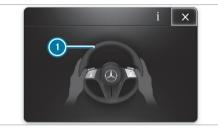
If the system detects that the driver has not steered the vehicle for a considerable period of time or has removed their hands from the steering wheel, an optical warning is given first. Display ① appears on the driver's display. If the driver still does not steer the vehicle, or gives no confirmation to the system, a warning tone sounds in addition to the visual warning message.
