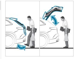
With HANDS-FREE ACCESS you can open, close or stop the closing process of the tailgate by performing a kicking movement under the rear bumper.
