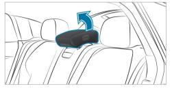
**To fold into position:** pull the head restraint upwards until it engages.
