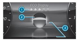
The ECO display shows an evaluation of your driving style on the driver's display depending on the situation. This enables you to check the efficiency of your driving style and adjust it if necessary. The ECO Display menu shows a ball (2) that will roll forwards or backwards on a stylized road in the direction of travel according to the driving characteristics.
