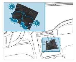
Manually push back the side walls of cup holder ② in the direction of the arrow.
