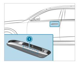
Unlocking the vehicle: with the door handle extended, touch the inside surface of door handle ().
