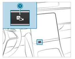
Press button ①. The Camera & Parking view opens in the central display.
