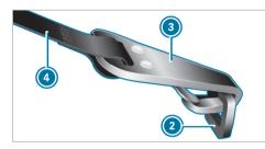
Guide Top Tether belt (4) under head restraint
