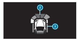
Optionally, obstacles detected by Parking Assist PARKTRONIC from a distance of approximately 3.3 ft (1.0 m) in front 2 and 2.0 ft (0.6 m) on the sides (3) can also be displayed in the head-up display.
