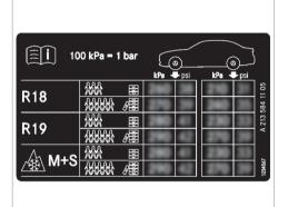
Some tire pressure tables only show the rim diameter instead of the complete tire size, e.g. R18. The rim diameter is part of the tire size and can be found on the tire side wall ( $\rightarrow$  page 368).
