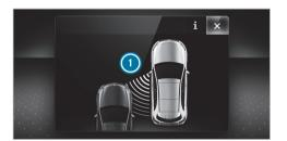
If a course-correcting brake application occurs, the red warning lamp will flash in the outside mirror and a warning tone will sound. In addition, display indicating the danger of a side collision will appear on the instrument display.
