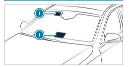
Radio-controlled equipment such as toll systems can be mounted only on areas (1) of the windshield that are permeable to radio waves.
