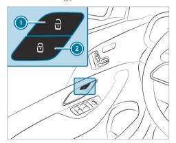
➤ To activate: press and hold button ② for approximately five seconds until an acoustic signal sounds.
