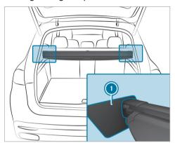
Insert the cargo compartment cover in brackets on the left and right.
