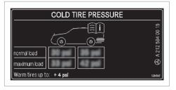
The tire pressure table shows the recommended tire pressure for all tires approved for this vehicle. The recommended tire pressures are valid for cold tires under various operating conditions according to the load and/or speed of the vehicle.
