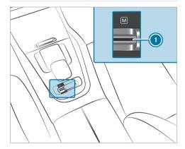
To activate/deactivate: pull rocker switch (1). If the indicator lamp is lit, manual shifting is activated. The current gear will be displayed on the Instrument Display.
