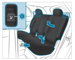
To fold the seat into the front position: briefly pull on button 1.
