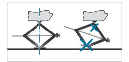
Rules of conduct when the vehicle is raised:
