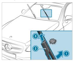
To bring the wiper blade into position to be removed: hold the wiper arm firmly with one hand. With the other hand, turn the wiper blade in the direction of arrow beyond the point of resistance.
