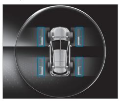
You can display the current distribution of drive torque to all four wheels on the head-up display and in the right-hand display range of the Instrument Display. The fuller the respective scale, the higher the corresponding drive torque.
