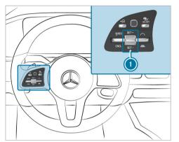
To operate Active Distance Assist DISTRONIC: press the rocker switches on the steering wheel control unit up or down to the desired position.
