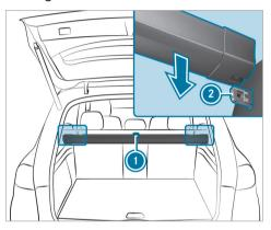
With tab (1) facing backwards, push the partitioning net cassette into brackets (2).
