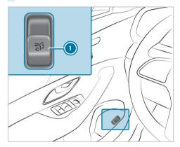
Pull remote operating switch until the tailgate opens.
