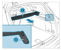
Pull the cargo compartment cover back by grab handle 1 and hook it into brackets 2 on the left and right.
