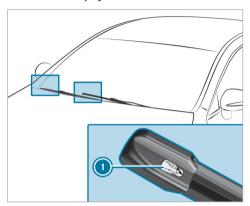
Remove protective film (1) from the maintenance displays on the tips of the newly installed wiper blades.
