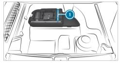
Towing eye 1 is located under the cargo floor by the tire-change tool kit.
