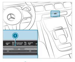
Indicator lamp  $\bigcirc$  flashes when the ATA system is armed.
