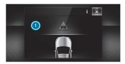
If autonomous braking or situation-dependent braking assistance has occurred, indicator 1 will appear on the instrument display and then automatically go out after a short time.
