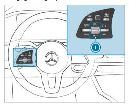
To increase/reduce the target speed: press rocker switch (1) up SET/+ or down SET/- to the point of resistance.
