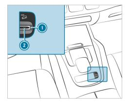
To activate: pull rocker switch 1. Indicator lamp 2 lights up. The symbol appears in the multifunction display.
