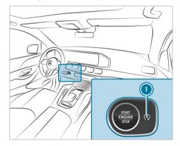
Press button ①. A display will appear on the instrument cluster when you switch the ECO start/stop function on/off. (i) 🔊 will be continuously shown on the instrument cluster while the ECO start/stop function is deactivated.
