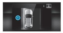
If a lane-correcting brake application occurs, display will appear on the instrument display.
