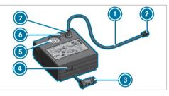
Pull filler hose ① and plug ③ out of the tire inflation compressor housing.
