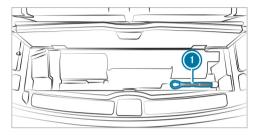
Towing eye 1 is located under the cargo floor.
