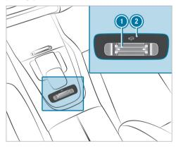
Push rocker switch ① forwards. Indicator lamp ② flashes while the vehicle is being raised and lights up continuously when it has finished rising.
