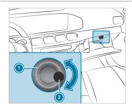
To open or close: turn controller of air vent clockwise or counter-clockwise.
