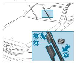
Push the new wiper blade onto the wiper arm in the direction of arrow 1 until release knob engages.
