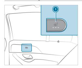
Seat heating in the rear passenger compartment
