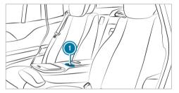
Mat in front of the stowage compartment in the rear passenger compartment armrest
