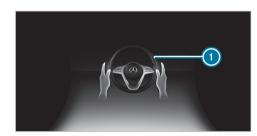
If the system detects that the driver has not steered the vehicle for a considerable period of time or has removed their hands from the steering wheel, display appears. If the driver still does not steer the vehicle, a warning tone sounds in addition to the visual warning message.
