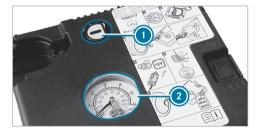
To reduce the tire pressure: press pressure release button 1 next to manometer 2.
