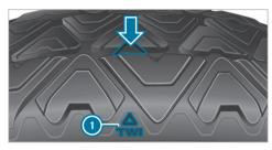
Six marks 1 show where the bar indicators (arrow) are integrated into the tire tread. They are visible once a tire tread depth of approximately 1/16 in (1.6 mm) has been reached.
