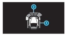
Optionally, obstacles detected by Parking Assist PARKTRONIC from a distance of approximately 3.3 ft (1.0 m) in front ② and 2.0 ft (0.6 m) on the sides ③ can also be displayed in the head-up display.
