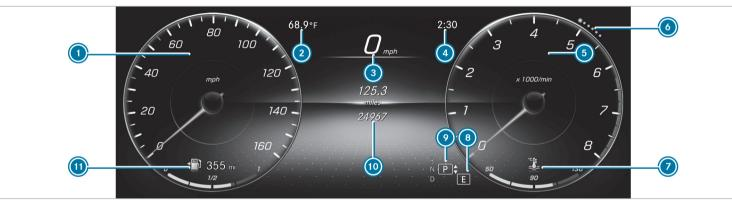
Left display area of the instrument display (example: speedometer): speedometer/time/ date/trip computer From Start and From Reset/range/audio/angle of incline and approach
