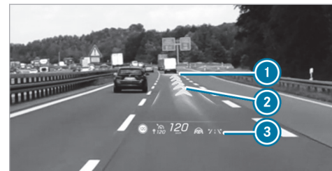
Head-up display with augmented reality (example)
