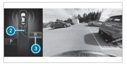
Parking spaces detected by the system are shown in the media display. When the vehicle is stationary, indicated vehicle path (2) into currently selected parking space (3) also appears.
