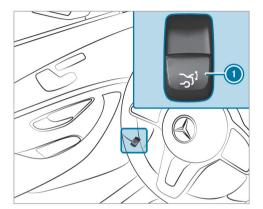
Pull remote operating switch ① until the tailgate opens.
