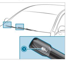
Remove protective film () from the maintenance displays on the tips of the newly installed wiper blades.
