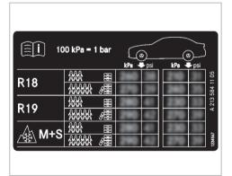
Some tire pressure tables only show the rim diameter instead of the complete tire size, e.g. **R18**. The rim diameter is part of the tire size and can be found on the tire side wall ( $\rightarrow$  page 339).
