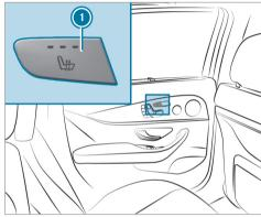
Press button ① repeatedly until the desired heating level is set.
