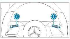
When the automatic transmission is shifted to position  $\boxed{\mathbf{D}}$ , you can manually shift it with the steering wheel gearshift paddle. If permitted, the automatic transmission shifts to a higher or lower gear depending on the steering wheel gearshift paddle being pulled.
