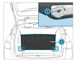
To remove: fold seat cushion (2) vertically upwards and remove it from seat cushion guide (1). Installing
