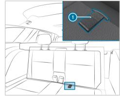
Pull the seat cushion upwards by tab () and fold it back into its starting position until it engages.
