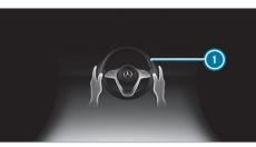
If the system detects that the driver has not steered the vehicle for a considerable period of time or has removed their hands from the steering wheel, display () appears in the Instrument Display. If the driver still does not steer the vehicle, or gives no confirmation to the system, a warning tone sounds in addition to the visual warning message.
