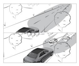
Adaptive Highbeam Assist Plus automatically switches between the following types of light:
