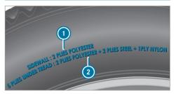
(i) The data shown in the image is example data. This information describes the type of tire cord and the number of layers in side wall (1) and under tire tread (2).
