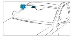
Radio-controlled equipment, e.g. toll systems, can be mounted only on areas of the windshield that are permeable to radio waves ().
