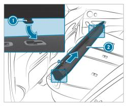
Insert combined cargo cover and net ② into both guides ③ and push it as far as it will go in the direction of the arrow.
