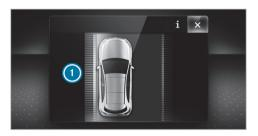
If a lane-correcting brake application occurs, display (1) appears in the Instrument Display.
