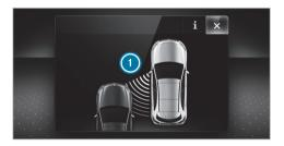
If a course-correcting brake application occurs, the red warning lamp flashes in the outside mirror and a warning tone sounds. In addition, display () indicating the danger of a side collision appears in the Instrument Display.
