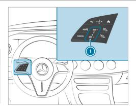
Steering wheel control panel for cruise control
