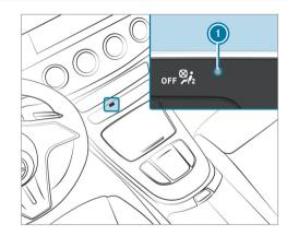
Indicator lamp 0 flashes when the ATA system is armed.
