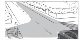
The cornering light improves the illumination of the road over a wide angle in the turning direction, enabling better visibility on tight curves, for example. It can be activated only when the low beam is switched on.
