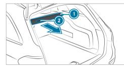
To extend: pull cargo compartment cover back by handle and clip it into the brackets on the left and right.
