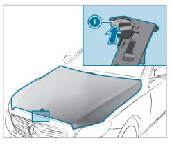
Push handle ① of the hood catch upwards and lift the hood until it opens automatically.
