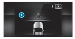
If autonomous braking or situation-dependent braking assistance has occurred, display () appears in the Instrument Display and then automatically goes out after a short time.  WARNING Risk of an accident caused by limited detection performance of Active Brake Assist
