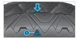
Six marks O show where the bar indicators (arrow) are integrated into the tire tread. They are visible once a tire tread depth of approximately  $\frac{1}{16}$  in (1.6 mm) has been reached.
