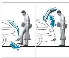
With HANDS-FREE ACCESS you can open, close or stop the closing process of the tailgate by performing a kicking movement under the rear bumper.
