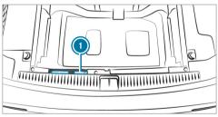
Towing eye () is attached to the edge of the cargo compartment under the cargo compartment floor.
